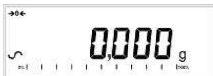
A stable sign ~ is shown when the balance is in stable condition. It will turn off if the balance is not stable.
