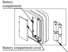
Remove the battery compartment cover and insert six batteries(R6P/LR6 /AAsize) into the battery compartment, taking extreme care that the polarities plus and minus is observed.
