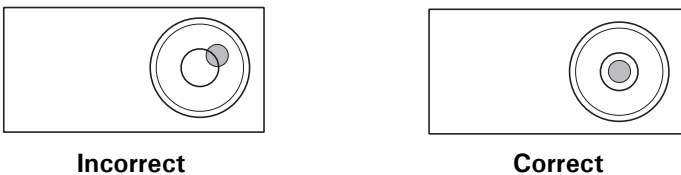
Fig. 3.2 Correct levelling with the aid of the bubble level
