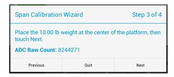
Wait for the Scale System to collect the data for the known weight.
