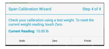
If the Front Panel is showing a value other than the test weight, remove the test weight from the platform, then press the ZERO button, and then try placing the test weight again on the platform.
