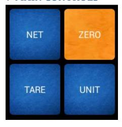
TARE Pressing this key will tare any weight on the platform and switch the scale to the net mode. Holding this
