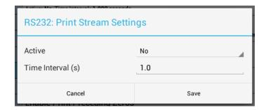
When stream mode is enabled, use the print button or the external ~\*P\*~ command to start or stop the printing process. You can easily toggle Print Stream by using the ON/OFF button located at the Option Selection.
